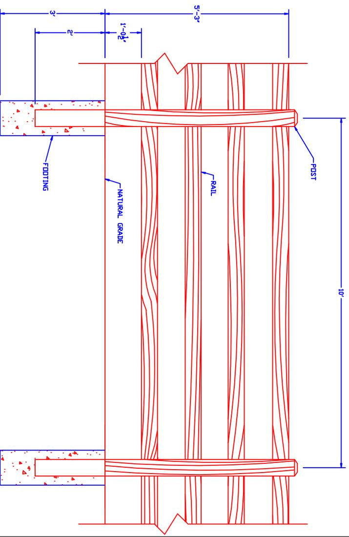
**4 RAIL 10 FT. SPACING FENCE ELEVATION**
